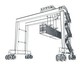
TCDS integrates computer vision models with crane control logic to ensure safe container handling during hoisting. It automatically detects the presence of twist-lock cones on containers before they're hoisted. Whether you're running RTGs, ARMGs, or other crane configurations, TCDS helps operators avoid dangerous lifts caused by unremoved locking devices.
