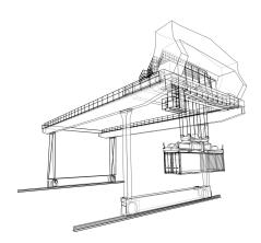
TLPS combines Al-powered computer vision with crane control logic to detect and prevent accidental lifting of trailers or chassis during container offloading. By monitoring the container-trailer interface in real time, TLPS ensures hoisting only begins when the container is safely disengaged—helping prevent dangerous lifts caused by locked chassis across RTGs, ARMGs, and other crane types.
